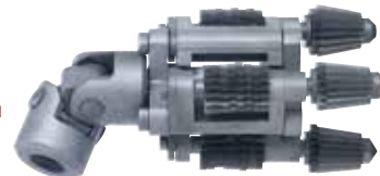
TYPE-5 Wing Arm Head with Universal Joint Range: 1-3/4 in. (44.4 mm) - 13-1/4 in. (336.5 mm) Self feeding Deposit: 1/2 in. (12.7 mm) - thick-hard to medium
