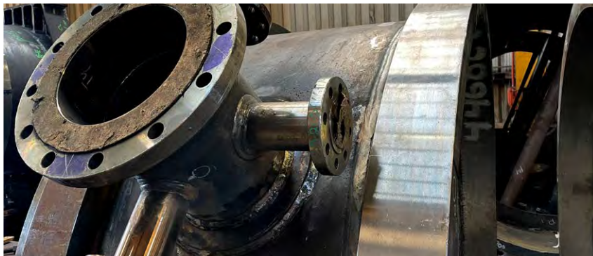
Example of really tight flange – NBBF is the only tool suitable here.
