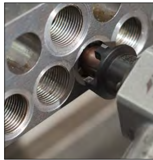
Safely re-machine gasket surfaces in seconds.
