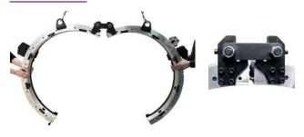
Accessory for convenient folding and unfolding of the device. It also allows the use of cranes and lifts that make work easier.
