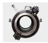
Out of round tool slides - can be solution for all misshapen tubes and pipes. Out of round slides feature durable springs and tracking module that follows the contours of a deformed or less than perfectly round pipe. Built with the same quality: for strength and durability as other KRAIS tool slides.
